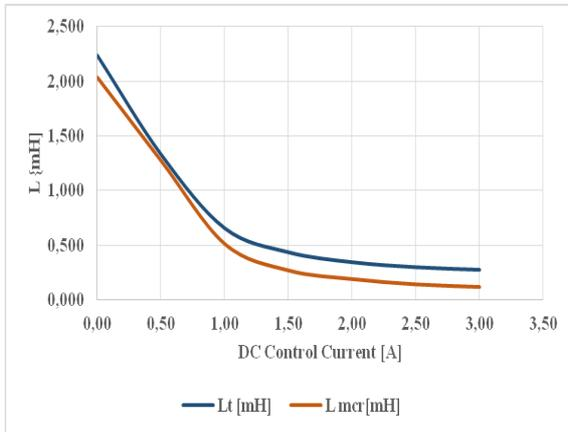
Fig. 2. Inductance variation with the DC control current.
