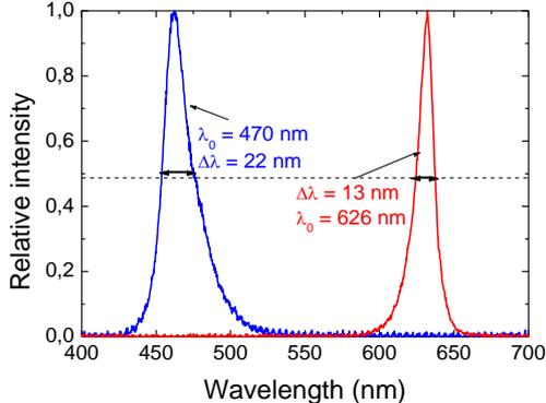
Fig. 3. Output spectra of the red and blue chips.
