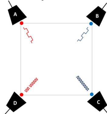
Fig. 1. Configuration of the experimental setup showing the position of the white LEDs and the wavelength and frequency of the modulation chip..
