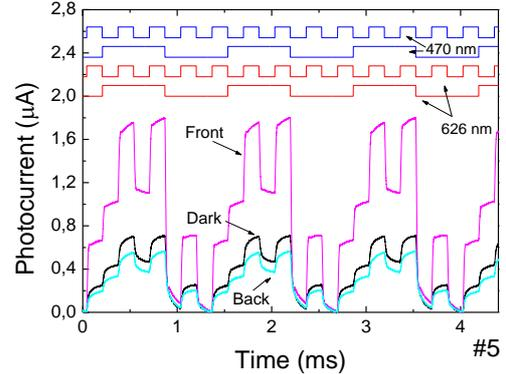
Fig. 4. Photocurrent measured without and under front and back optical bias when the device is at the central position.
