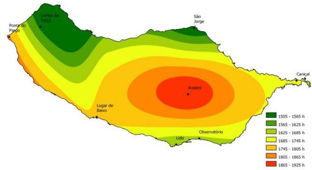
Figure 4 - Equivalent sun hours at peak power in Madeira.
