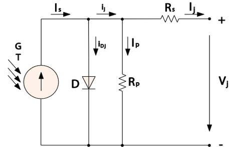
Figure 1 – Equivalent circuit of a solar cell.
