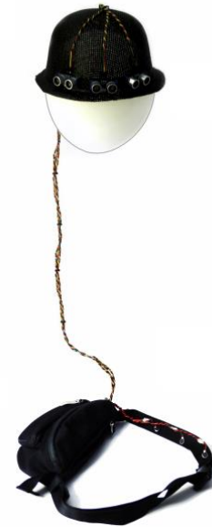
Fig. 1. Developed system for object detection for blind users. It is composed of three main modules: sonar module, user interface module, and a signal processing module.
