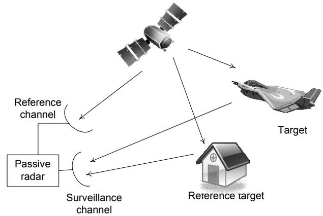
Fig. 2. Passive bistatic radar acquisition geometry using a reference target to correct the signal phase.
