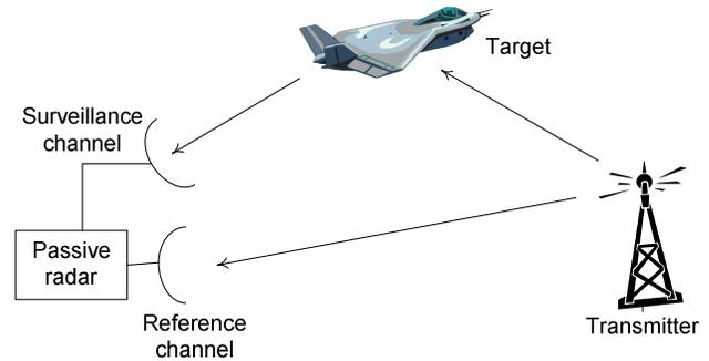
Fig. 1. Passive bistatic radar acquisition geometry. Direct signal from the transmitter is reflected on a given target. The receiver antenna processes both the direct and the reflected signal. These two signals exhibit high correlation between themselves..
