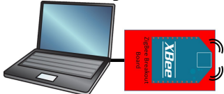
Fig. 3. ZigBee receiver diagram with Breakout Board.
