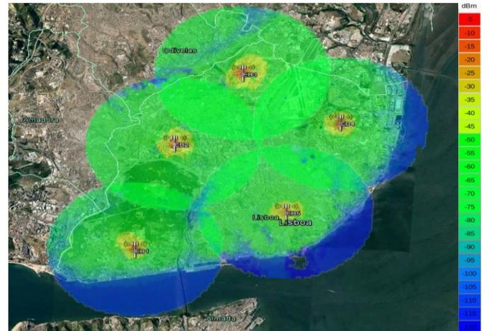
Fig. 3 – Coverage with model Okumura-Hata.
