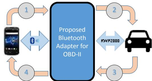
Fig. 3 - Block diagram of the system architecture.
